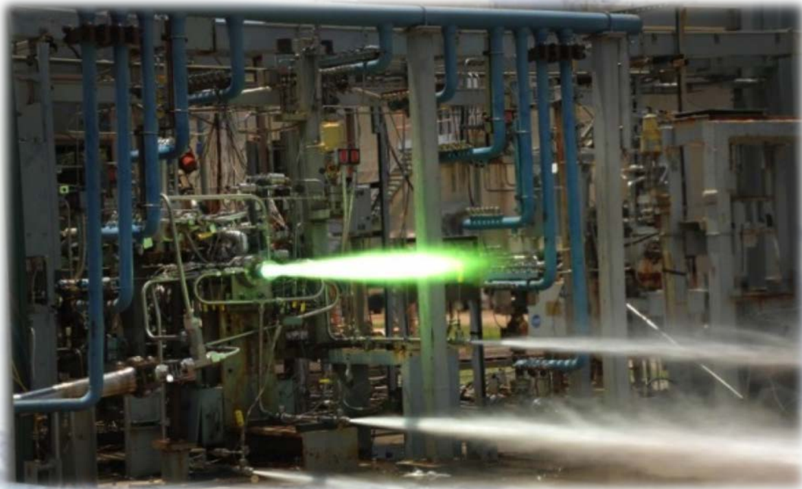
NASA Test-Firing a Rocket with 3D-Printed Components. Credit: NASA
